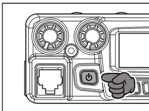
2. To turn the transceiver off, again press and hold in the **PWR** key for one second.
