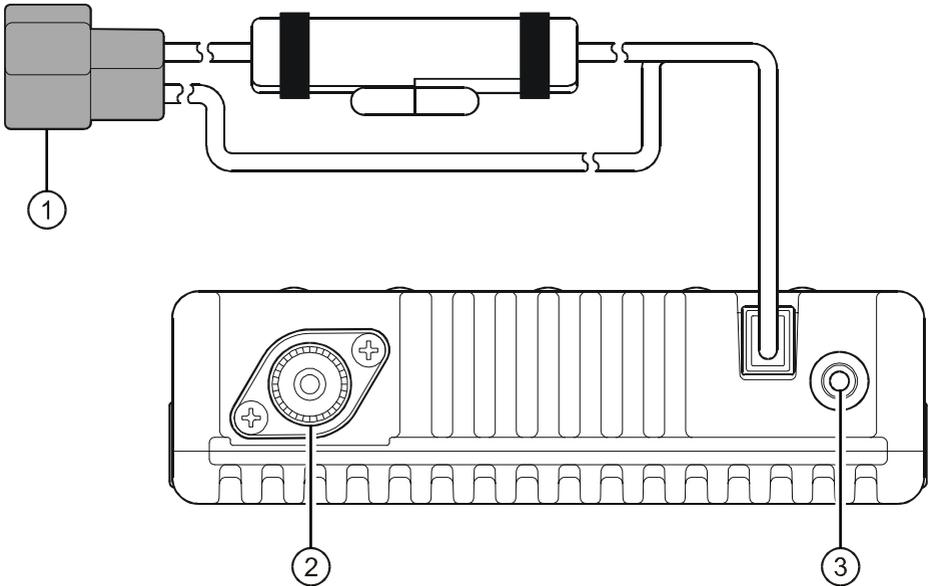
① **13.8V DC Cable Pigtail w/Fuse**
